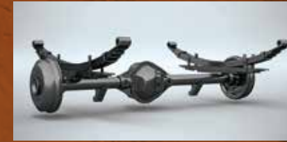
Strong 9 leaf suspension and double bearing axle
